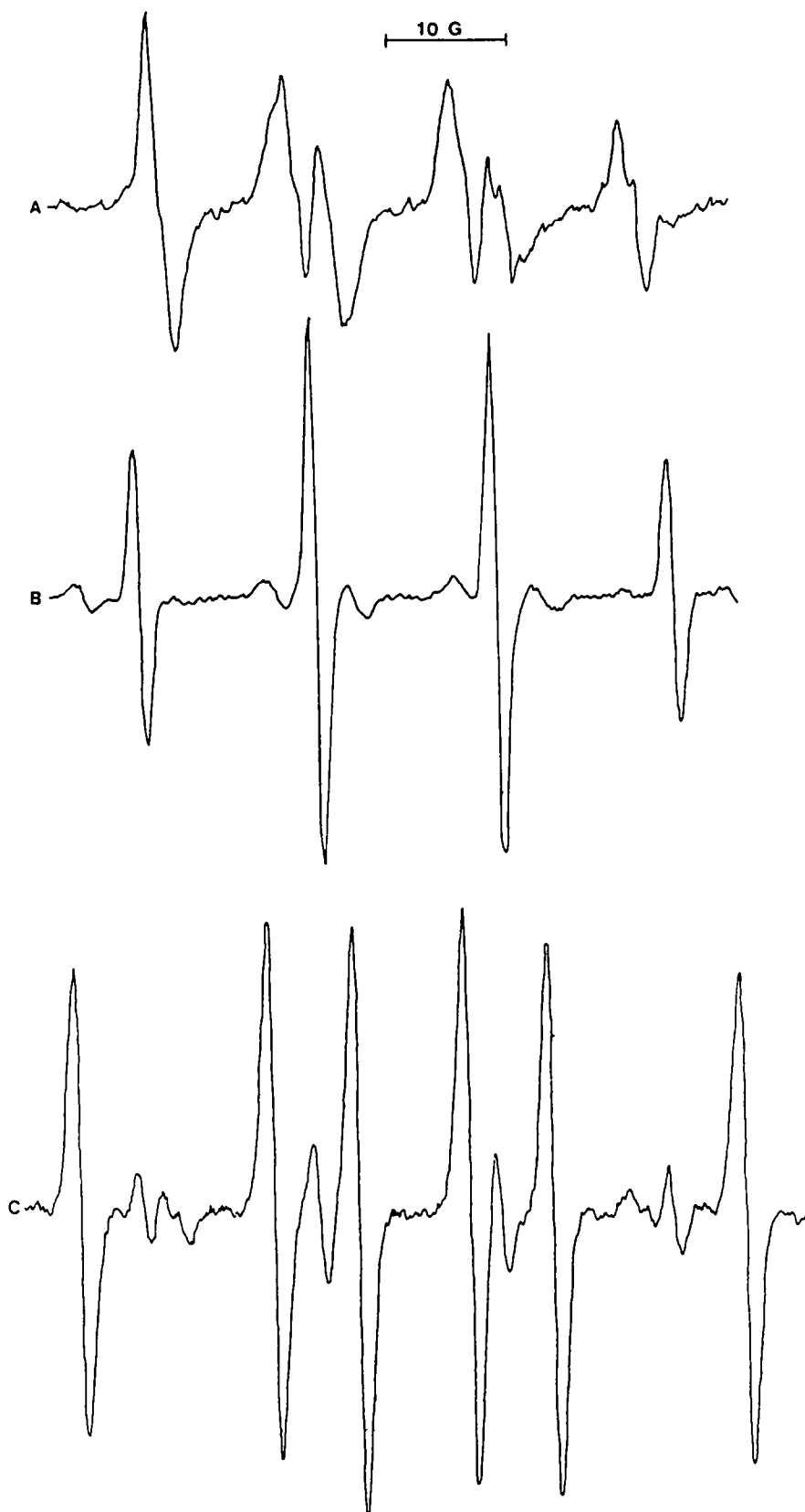
Fig. 2. (A) ESR spectrum obtained from a superoxide-generating system consisting of hypoxanthine and xanthine oxidase in the presence of DMPO (0.1 M). A_N = 14.3 G and A_H = 11.7 G. (B) ESR spectrum obtained when ferric ammonium sulfate (0.1 mM) was added to the aforementioned superoxide-generating system. A_N = A_H = 14.9 G. (C) ESR spectrum obtained when DMSO (0.14 M) was added to B. A_N = 15.3 G and A_H = 22.0 G. The microwave power was 20 mW and the modulation frequency was 100 kHz with an amplitude of 1.0 G. The sweep time was 12.5 G/min and the receiver gain was 8.0 \times 10^3 with a response time of 1.0 sec.
